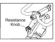
To stop the flywheel, push the resistance knob downward. The flywheel should quickly come to a complete stop.
